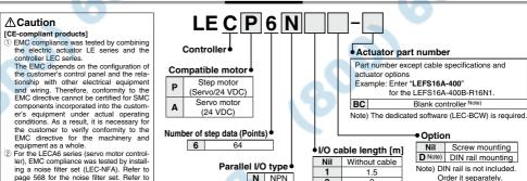
\* When controller equipped type is selected when ordering the LE series, you do not need to order this controller.
