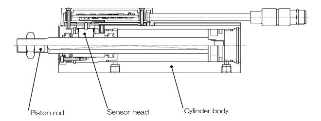
• A part of the piston rod has scale (magnetic scale). In order to maintain the relative position of the scale and the sensor head, piston rod is used to have a structure of non-rotating cylinder.
