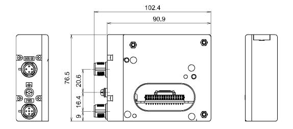
•If a fieldwireable connector is used for the power supply connection, and the SI unit is installed directly to a valve manifold, the connector should be  $\phi$ 16 mm or less.
