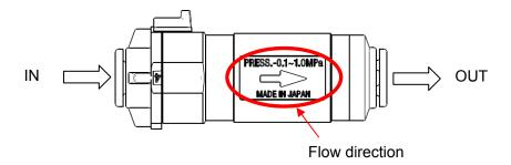
Note) When replacing the element, ensure that there is enough space for removing the cover (IN side). Note) Refer to "One-touch Fittings Precautions" for mounting and removal of the tube.
