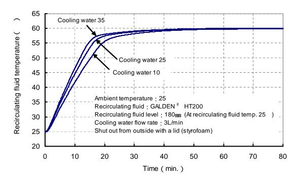
Fig. 7-5 Heating capacity
