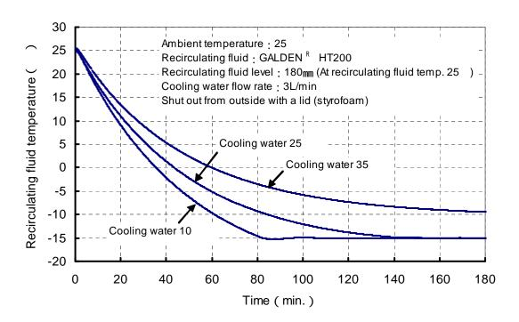
Fig. 7-4 Cooling capacity
