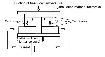
Fig. 3-2 Construction and principle of thermo-module
