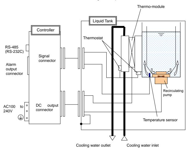
Fig. 3-3 Operation principle
