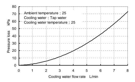
Fig. 7-6 Radiating water pressure loss
