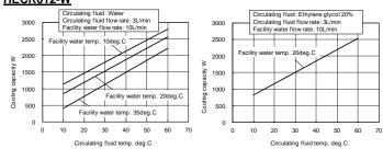
\*Cooling capacity decrease about 50W when high head pump option selected.
