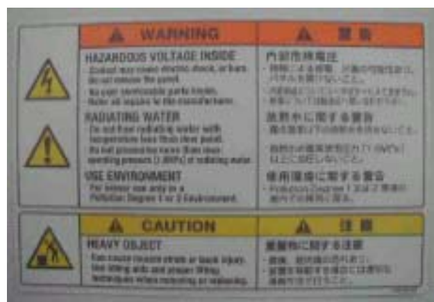
Fig. 2-2 Detail of “Warning” label and “Caution” label
