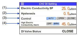
Electric conductivity and alarm (AL27) setting
