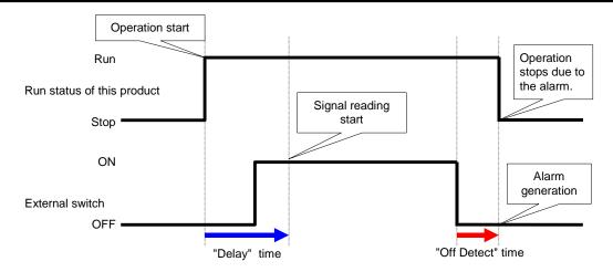
"Delay" time and "off detect" time
