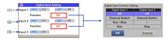
Setting of contact input signal form
