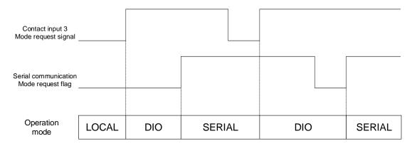
Fig.1-2 Mode switching by the mode request (ON state mixed)
