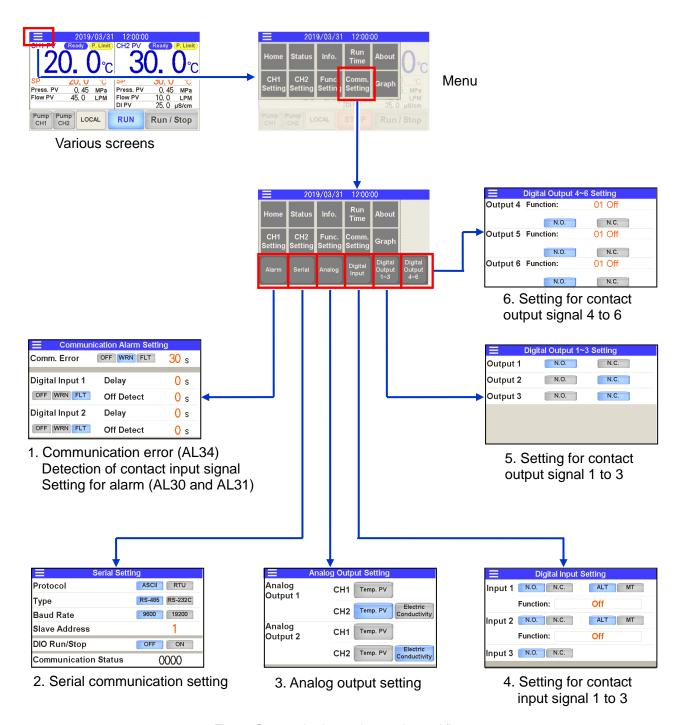
Fig.1-4 Communication setting touch panel flow
