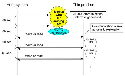
Fig. 4-2 Communication alarm restoration example
