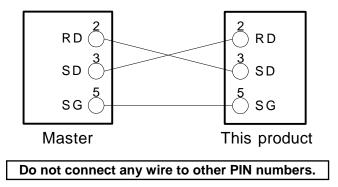
Fig 3-2 RS-232C connector connection
