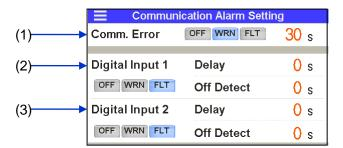
Communication error, detection alarme of contact input signal and setting
