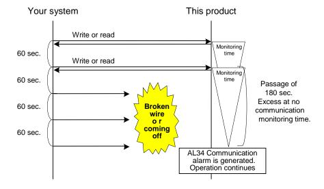
Fig. 4-1 Communication alarm example
