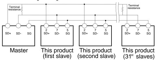
Fig 3-1 RS-485 connector connection
