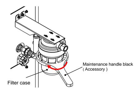
Fig. 3-21 CH2 particle filter case removal
