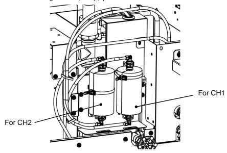
Fig. 7-5 Temporary pipe installation for DI filter(For option D1)
