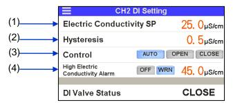
Electric conductivity and alarm (AL27) setting
