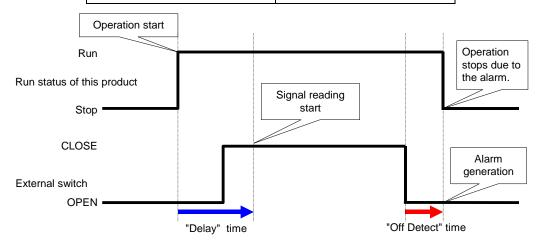
"Delay" time and "Off detect" time
