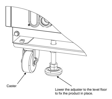
Fig. 3-5 Installation by adjuster foot
