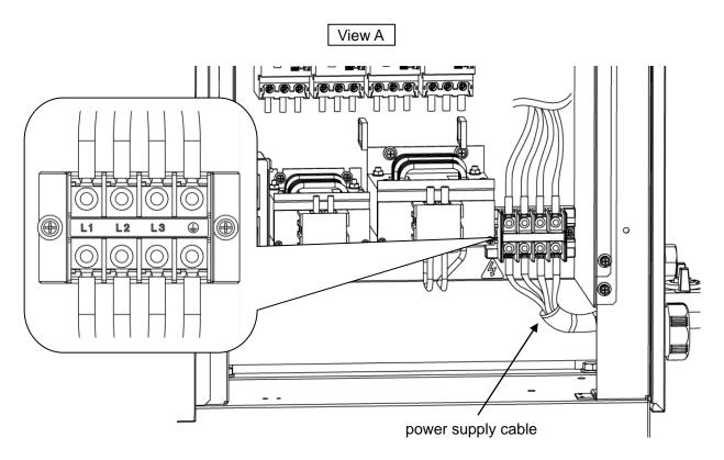
Fig. 3-9 Wiring of power supply cable
