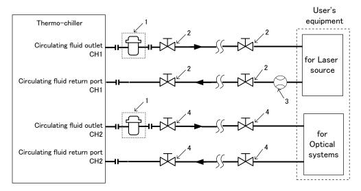
Fig. 3-24 Recommended piping circuit
