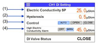
Electric conductivity and alarm (AL28) setting
