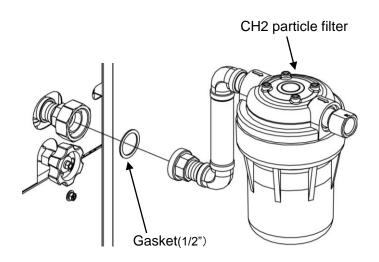
Fig. 3-18 CH2 side Installation of particle filter
