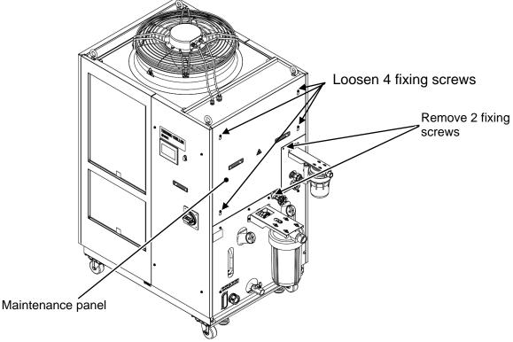
Fig. 7-6 Maintenance panel removal
