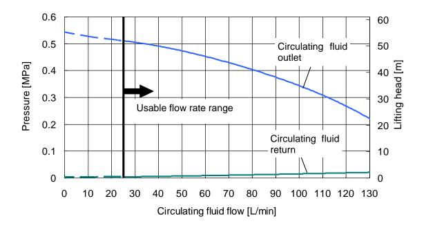
Fig. 8-10 Pump capacity(HRL200-A\*-40 CH1)
