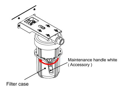
Fig. 3-20 CH1 particle filter case removal
