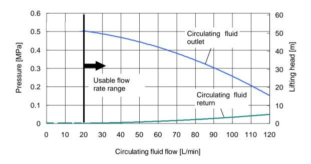
Fig. 8-9 Pump capacity(HRL100-A\*-40 CH1)
