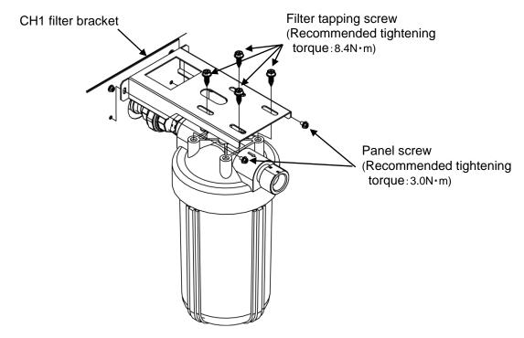
Fig. 3-16 CH1 side Installation of filter bracket.
