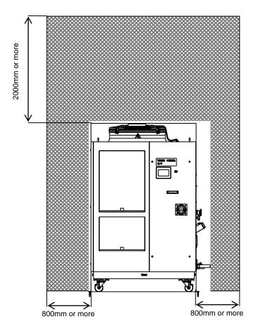
Fig. 3-3 Installation space (This drawing shows "HRL200-A-20".)
