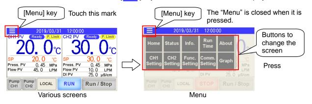
**3.** Press a button for example to carry out "Run/Stop," "Selection of function" or "Change the screen.
