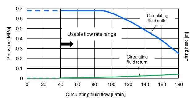
Fig. 8-11 Pump capacity(HRL300-A\*-40 CH1)
