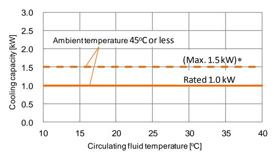
\*Up to 1.5kW.However,when 1.5kW heat load is applied,the cooling capacity of CH1 will decrease by 0.5kW.
