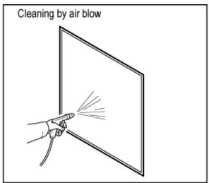
Fig. 7-2 Cleaning of the dust-proof filter
