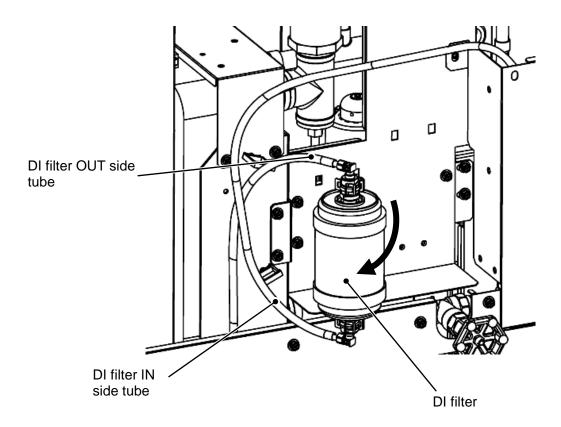
**5.** The connection fitting of the DI filter and the tube is connected by a fastener. O ring is used for the connection fitting. After removing the fastener, remove the connection fitting. Be careful not to apply force to the tube at this time. Also, please be careful not to damage the Oring.
