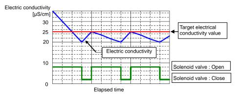
Fig.5-7 Example of electrical conductivity control
