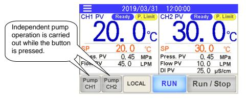
Fig.4-5 Pump independent operation
