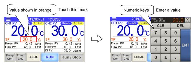
Fig. 4-8 Setting of CH1 circulating fluid temperature
