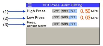
Setting of discharge pressure alarm (AL18/AL19/AL20)
