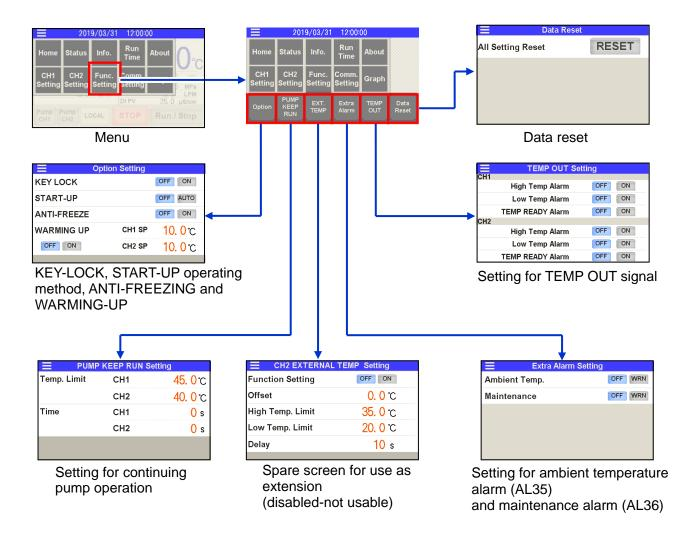
•KEY-LOCK, START-UP operating method, ANTI-FREEZING and WARMING-UP
