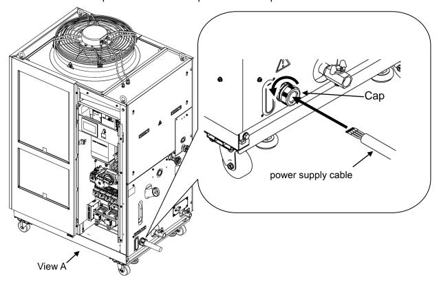
Fig. 3-8 Wiring of power supply cable
