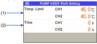
Setting for continuous pump operation
