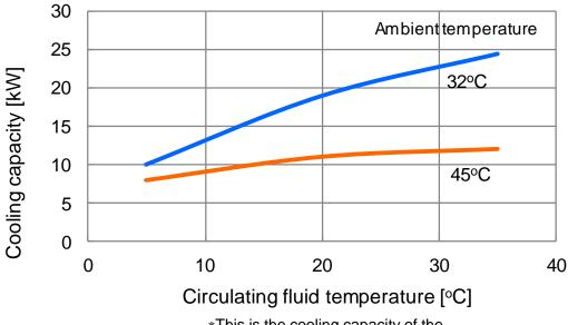
\*This is the cooling capacity of the CH1 side when 1 kW heat load is applied to the CH2 side.
