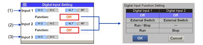
Setting of contact input signal form
