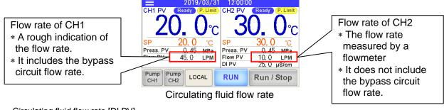
Circulating fluid flow rate [DI PV]
