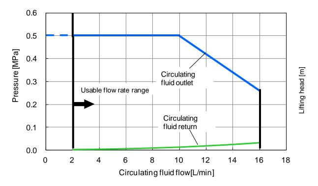
Fig. 8-12 Pump capacity(HRL100/200/300-A\*-40 CH2)
