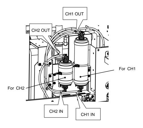
**4.** Pull out the DI filter to the front. The DI filter has been connected to the tube. Please allow excessive force is not applied to the tube.
