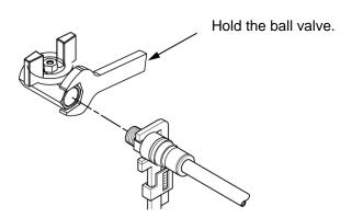
Fig. 3-23 Connection to the drain port
