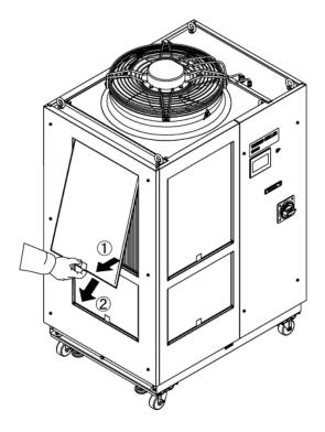
Fig. 7-1 Removal of the dust-proof filter
