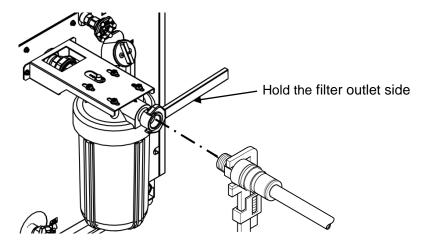
Fig. 3-22 Hold the filter outlet side
