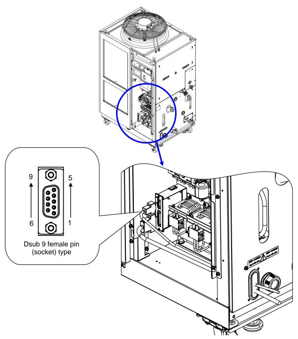
Fig. 3-12 RS-485 communication wiring
