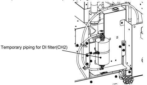
Fig. 7-4 Temporary pipe installation for DI filter
