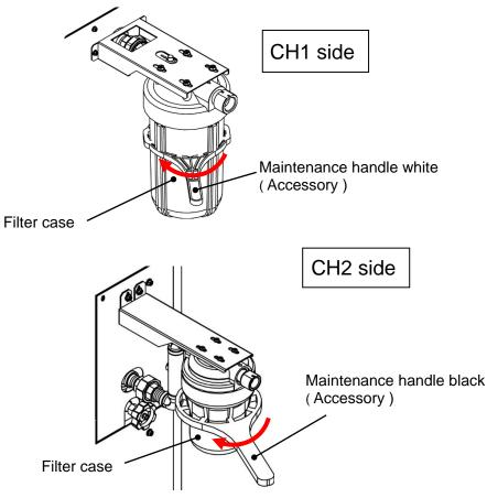
Fig. 7-3 Particle filter removal
