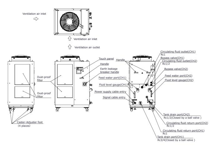
Fig. 2-2 Names of the parts (This drawing shows "HRL200-A-40".)
