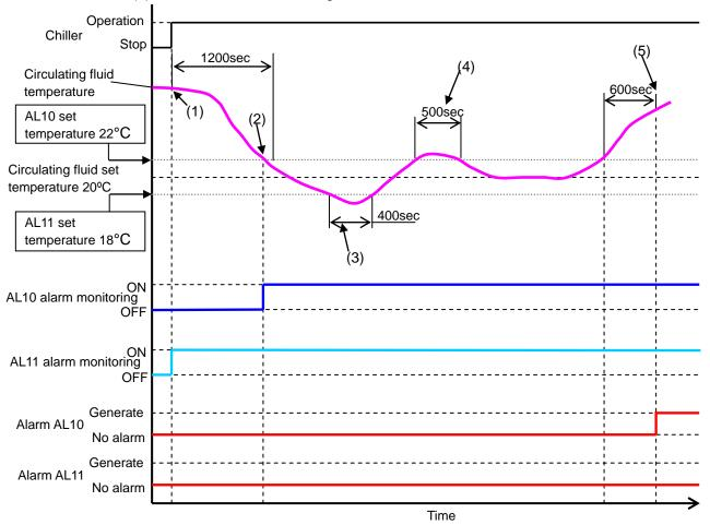
Fig. 5-5 Alarm monitoring timing
