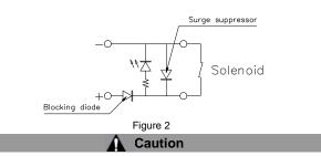
The surge suppressors fitted to the valve are intended to protect the output device so that the surge generated inside the valve does not affect the output device. External overvoltage or overcurrent might damage the surge suppressor, the valve and the output device itself. Additional safety measures should be taken to prevent the effect of overcurrent on the valve and connected devices.
