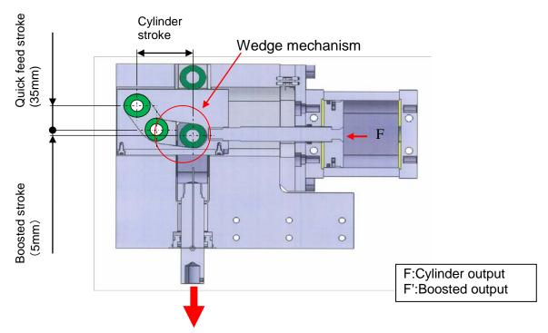
$F'=6\times F(When the stroke is boosted)$
