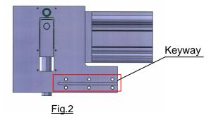
Rod end is shaped for slip fit. When mounting the unit to the rod end, fix using hexagon socket head set screws. If the rod end shape needs to be shaped other than for slip fit, please consult SMC.
