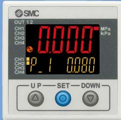
When the differential pressure reaches 0.08 MPa, a signal is output.
