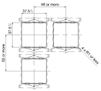
\*: Suitable for panel thickness of 0.5 to 8 mm. (When the waterproof seal is used, Suitable for panel thickness of 0.5 to 6 mm.)
