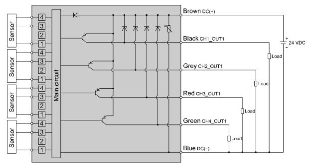
Max. 80 mA Internal voltage drop: 1.5 V or less
