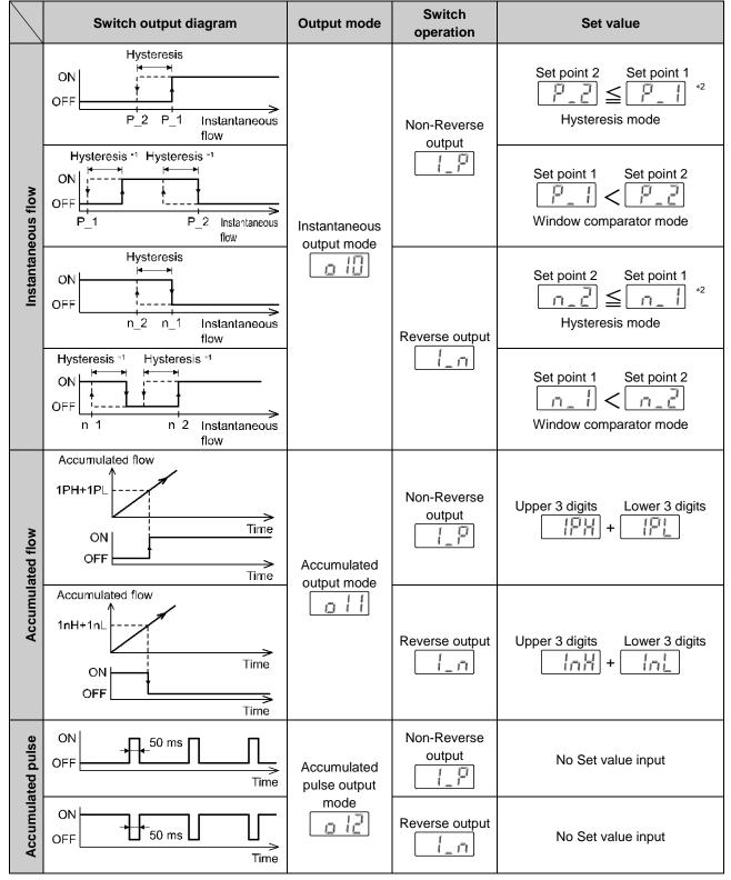
\*1: In window comparator mode, the hysteresis is fixed at 3 digits. When setting, allow 7 digits or more between Set point 1 and Set point 2. \*2: When Set point 1 = Set point 2, chattering may occur.
