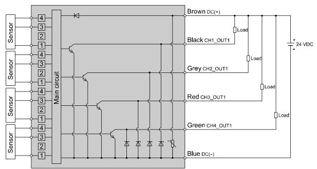
Max. 30 V, 80 mA Internal voltage drop: 1 V or less
