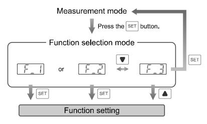
\*: When the output mode is set to instantaneous output mode, [F\_1] is displayed. When the output mode is set to accumulated output mode, [F\_2] is displayed. When the output mode is set to accumulated pulse output mode, [F\_3] is displayed.
