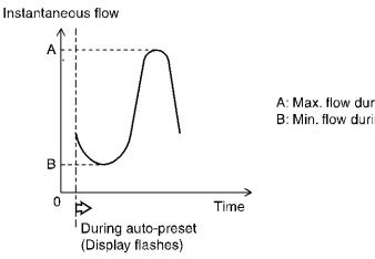
A: Max. flow during auto-preset mode B: Min. flow during auto-preset mode
