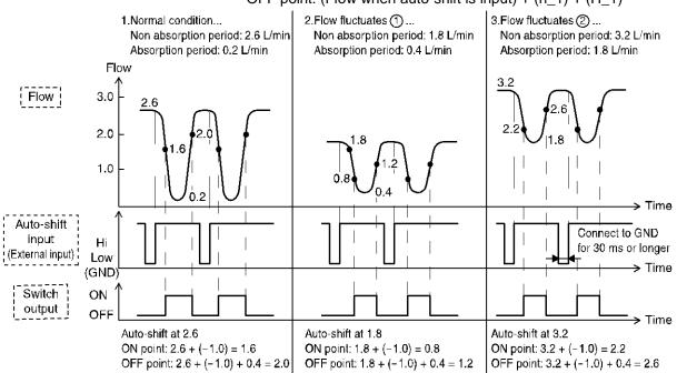
The table below shows an example of the flow displayed when auto-shift zero is selected. Here, a typical condition is used as an example
