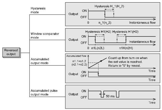
\*: If hysteresis or window comparator mode is selected and there is an unstable flow condition (due to fluid pulsation, for example), unstable output operation can result.
