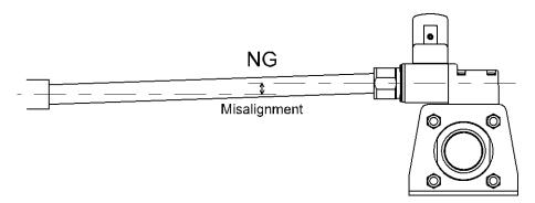
•When a flexible hose is used for the piping, the hose must be fixed with a bracket etc. If it is not fixed, the load weight of the flexible hose and the fluid will be applied to the product.
