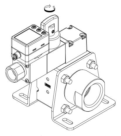
When closing and opening are repeated frequently, water leakage may occur due to wear of the internal seals.
