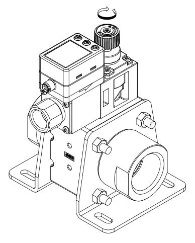
The flow adjustment valve is not designed for applications that require daily and repetitive adjustment. If the valve is adjusted frequently, fluid may leak due to wear of the internal seal.
