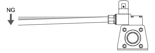
•Do not install piping to the product with a misalignment. A permanent load will be applied to the product after piping.
