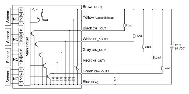
PSE201-(M)□: PNP open collector 5 outputs + Auto-shift 1 input
