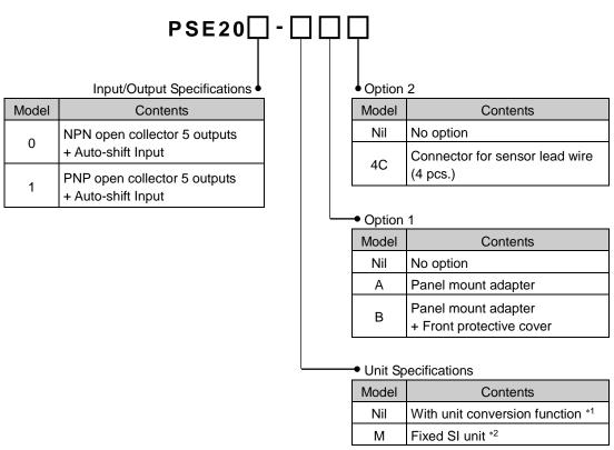
\*1: The new Measurement Law prohibits the use of pressure switch with the unit conversion function in Japan.
