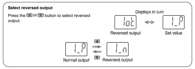
Press the S button to set. W Move on to setting of pressure.
