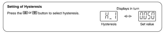
Press the S button to set. W Move on to setting of display colour.
