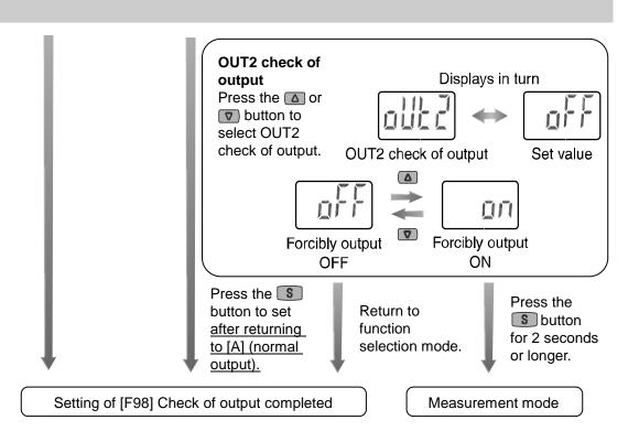
\*: If the \sigma\$ button is pressed for 2 seconds or longer, the mode is returned to measurement mode regardless of the current mode.
