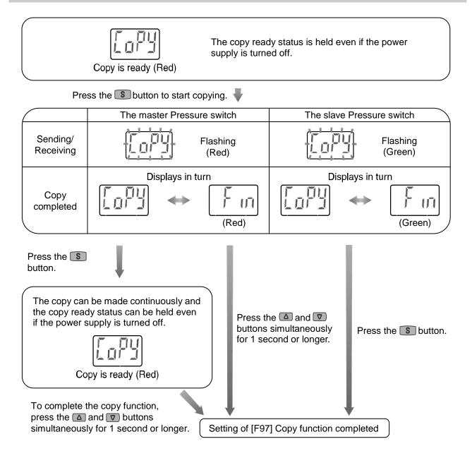
\*: If the copy to the slave pressure switch is not completed, it is detected as a copy function sending/receiving error.
