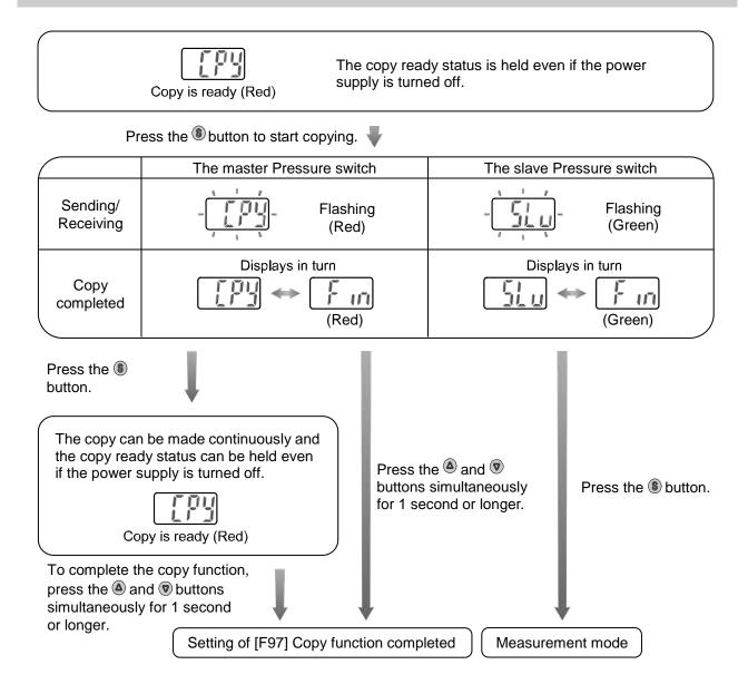
\*: If the copy to the slave pressure switch is not completed, it is detected as a copy function sending/receiving error.
