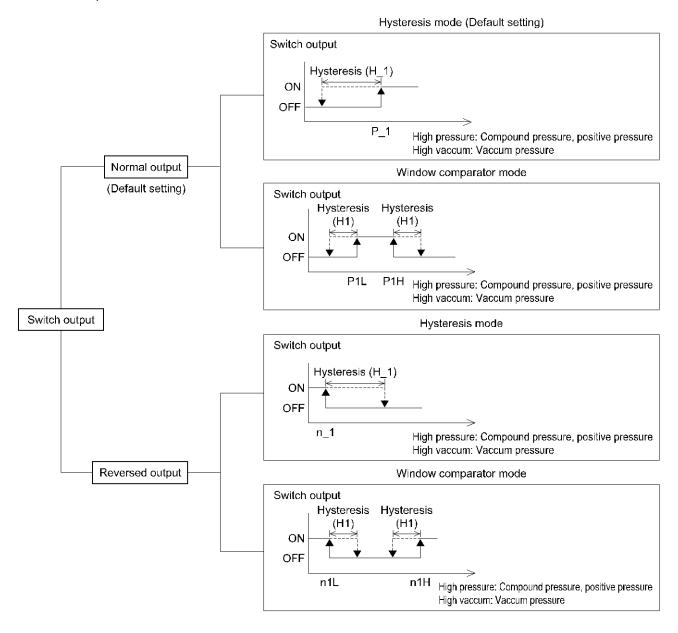
If the set value when the switch output is changed is outside the set pressure range due to switching between normal and reversed output, the hysteresis will automatically be compensated.
