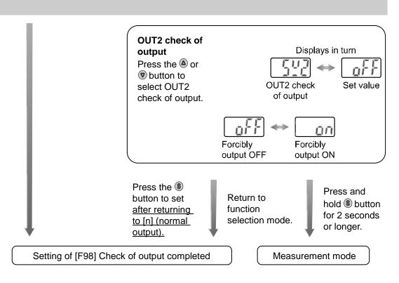
\*: If the ® button is pressed for 2 seconds or longer, the mode is returned to the measurement mode regardless of the current mode.
