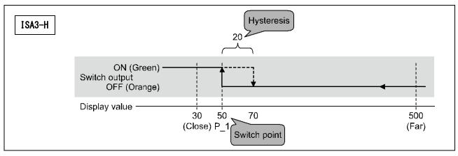
The switch output turns ON when the display value is less than switch point. (Solid line in the chart) The switch output turns OFF when the display value is greater than the switch point added to the hysteresis value. (Dashed line in the chart)
