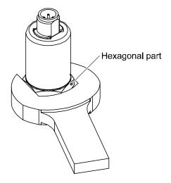
•When piping, apply a spanner to the piping section of the sensor.
