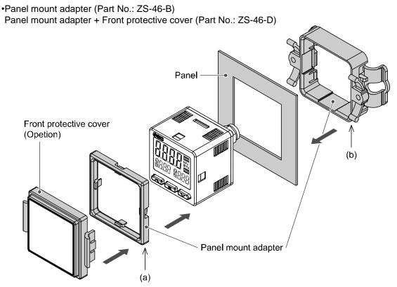
\*: The panel mount adapter can be rotated through 90 degrees for mounting.
