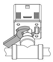
When tightening, do not hold the pressure switch body with a spanner.
