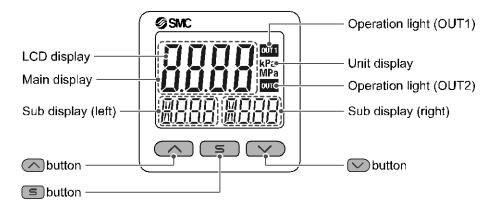
Operation light: Displays the switch operating condition.
