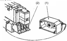
• The following marking are on the terminal block. Connect with corresponding power side.
