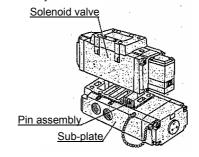
Tightening Torque for Mounting Bolt: 1.4N·m
