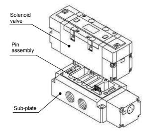
Tightening Torque for Mounting Bolt: 16 N·m
