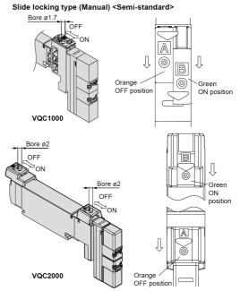
The manual override is locked by sliding it all the way to the pilot valve side (ON side) with a small flat head screwdriver or with your fingers. Slide it to the fitting side (OFF side) to release it. In addition, it can also be used as a push type by using a screwdriver, etc., of ø1.7 or less. (ø2 or less for VQC2000)
