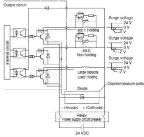
Figure 2. Surge Intrusion circuit example (NPN outlet example)
