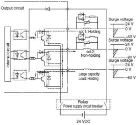
Figure 1. Surge intrusion circuit example (NPN outlet example)
