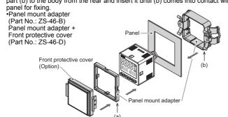
The panel mount adapter can be rotated through 90 degrees for mounting
